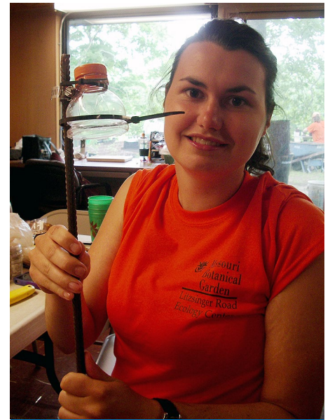
Chelsea Pretz holding a home-made mounting device for temperature sensors. Photo by Danelle Haake.
