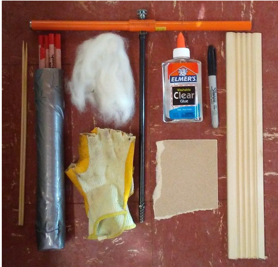
Figure 5. The tools used for this project from left to right: wooden skewers, straws in a paper towel tube, wool roving, gloves, increment borer, water soluble glue, permanent marker, sandpaper, wooden fluted trim to mount the cores.
